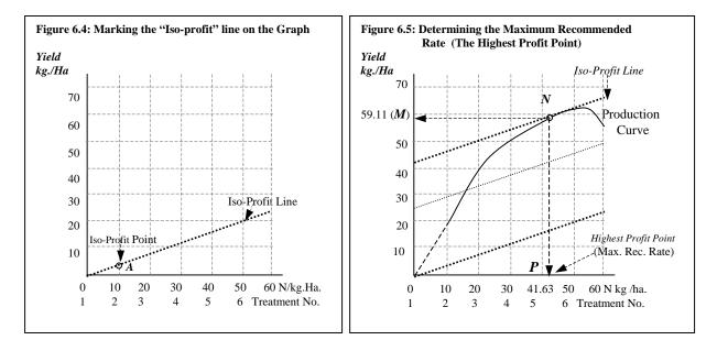
Now draw a straight line passing through point A and the axis  $\theta$ . This gives us the line OA. Now take a ruler and move the ruler parallel to the line OA, until the ruler is tangent to the production curve. When the line is tangent ( i.e has only one point of contact) to the production curve, we have found our *"iso-profit"* line.
